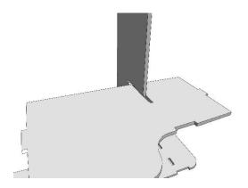
Take panel E and slot into panel B as shown in picture.
