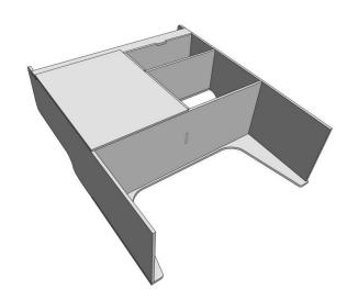
Place one of the back panel s (panel H) flush with the bottom shelf as per picture. Screw into place.
