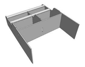
Lay the unit on its back. Take panel G (x2) align with end panels and screw into place.
