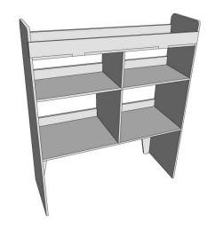
Insert panel J into the available slots as per picture. Screw into place.
