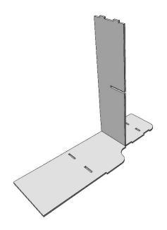
Take panel B and place into middle slots of panel A, as in picture.
