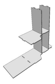
Take panel C and slot in to top slots of panel A (making sure front and rear edges are aligned if not, turnover) now slot onto panel E as shown.
