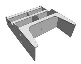
Take panel F, align with end panels and screw in to place.
