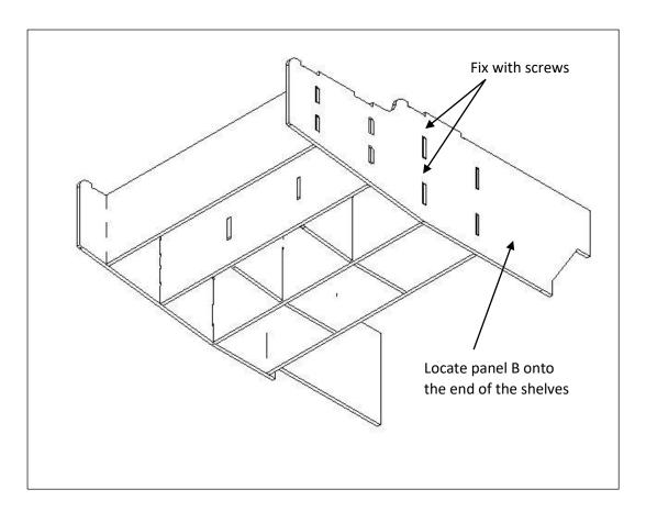
Carefully turn the unit over, trying to not let the other end panel fall off. Secure other end panel with screws.
