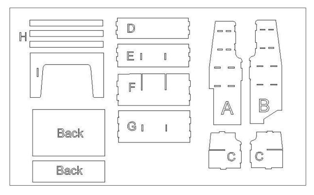
Note this unit is designed to work on either side of the van. Looking at the unit from the front if fitting to the drivers side of the van make sure panel "A" is on the left hand side. If fitting to the nearside of the van make sure that Panel "A" is on the right hand side of the unit. The following instructions are based on assembling a unit for the passengers side of the van. Swap panels A + B around if intending to fit on driverside.
