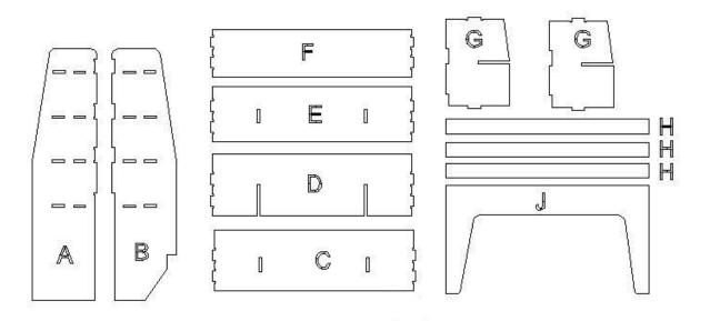
Note this unit is designed to work on either side of the van on top of the wheel arch. Looking at the unit from the front if fitting to the driver side of the van make sure panel B is on the left-hand side. If fitting to the nearside of the van make sure that Panel B is on the right hand side of the unit.
