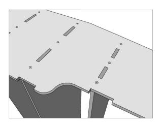
Take panel F and fit it into the remaining slots in the end panel.
