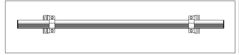
Once in position, tighten all fixings to **8Nm**. Periodically check all fixings.
