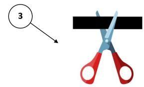
Cut the foam to length and stick to the bottom of the RRP77. Then, pierce through central hole.
