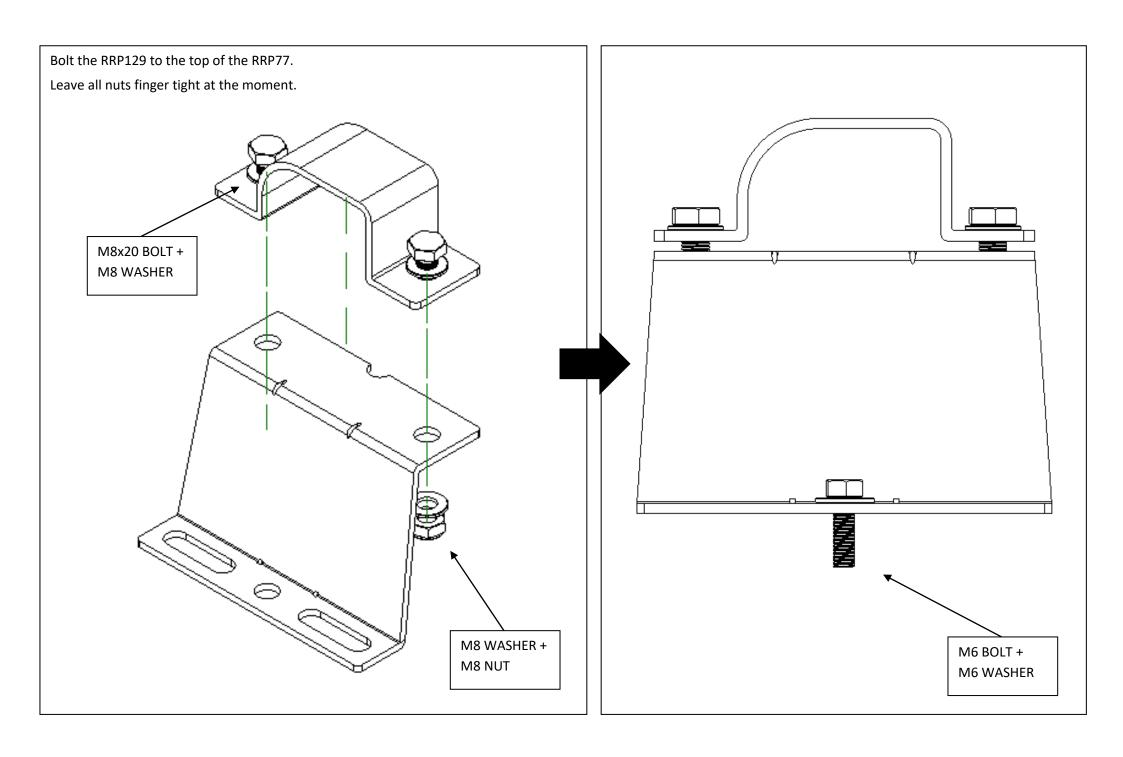
Slide the bar into place and make sure it is centrally positioned. At this stage, all nuts and bolts can be tightened.
