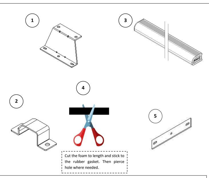
Note, there are 4 roof rack mounts on the roof of your van. This roof rack system has been designed that it can mount onto either the single bolt hole fixings or the twin bolt hole fixings.
