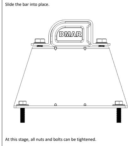
Once in position, tighten all fixings to **8Nm**. Periodically check all fixings.
