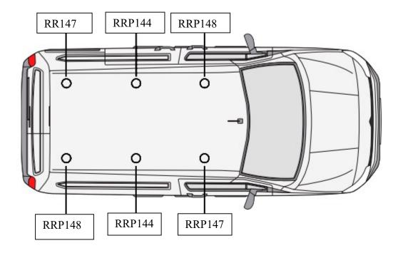
Brackets to be mounted on the roof in the positions detailed below.
